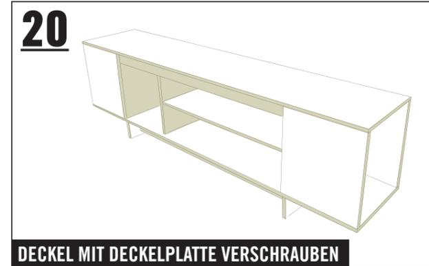
**20 DECKEL MIT DECKELPLATTE VERSCHRAUBEN**
