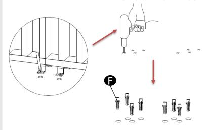
If the floor is a wooden floor, you don't need to knock in the plastic expansion pipe(REF F), use self tapping screw (REF E) to knock in the floor directly.
