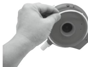
2. Use the screwdriver to unscrew the 4 screws located on the bottom of the head to release the bottom plate at first. Use the screwdriver to unscrew all the screws on the base as shown. Remove the impeller and then pry up the base and remove it to expose head inside.
