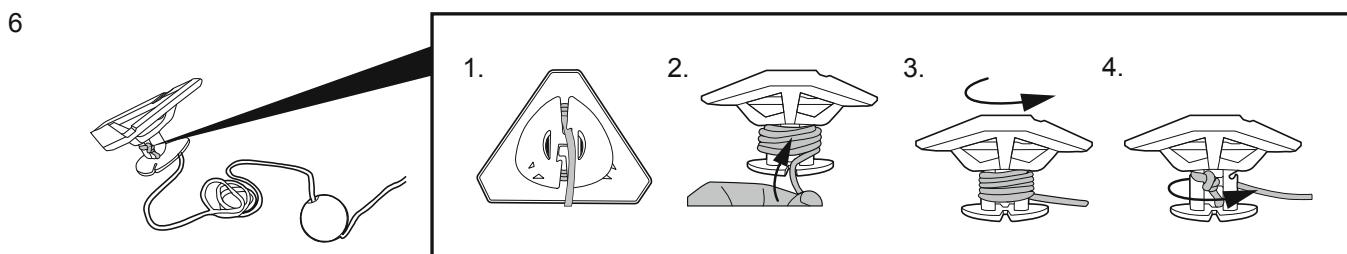
**Note:** Pry to detach the float cover and release the rope from the float to the depth of pool water plus about 0.5 m (19.7 in.).
