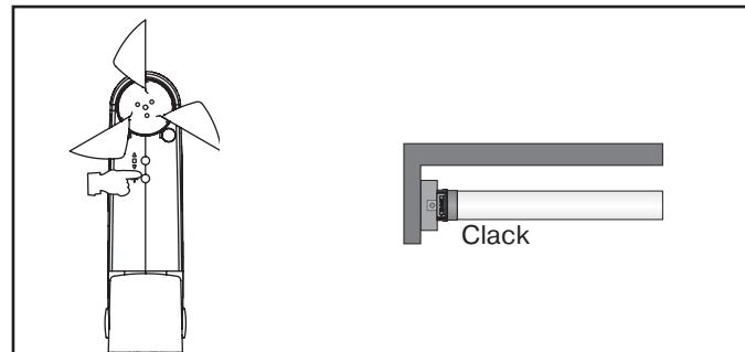
c) Now press again the programming button of the SC861 to be programmed until the tubular drive makes a „clack-clack“ sound to confirm.
