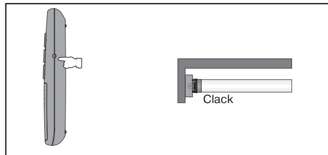
b) Now press the programming button of the SC861 until the tubular drive makes a „clack“ sound to confirm.
