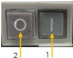
**Switch on:** Press the switch on button of the switch unit (1).
