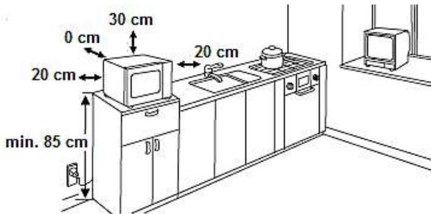
3. The back of the appliance must face a wall.
