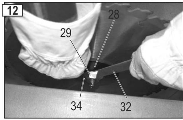
5. Now, the front saw blade flange (28) and the saw blade (27) can be removed.
