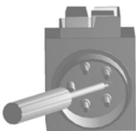
The rotating direction of three-phase motors can be changed by inserting a screwdriver in the connector collar provided for this purpose and turn left or right while exerting a light pressure to adjust the correct rotating direction.
