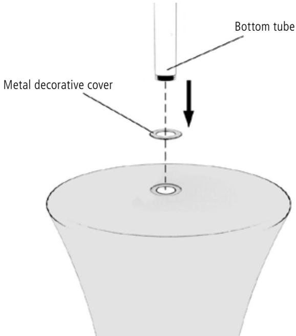
**Step 2:** Feed the power cord through the base and the bottom tube.
