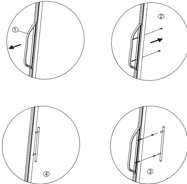
To do this, slide the rubber seal on the back of the door to the side to lay open the predrilled holes. Use the included screws to install the handle on the door.
