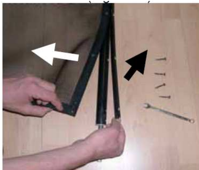
Fig. 11. Undo the 10 bolts of the fastening strip of the netting so the netting hangs free
