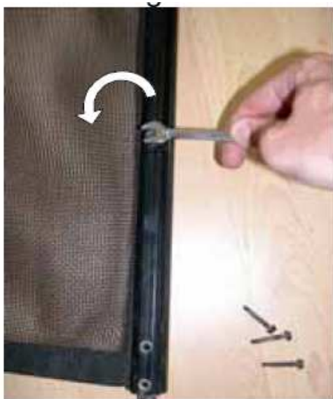
Fig. 11. Undo the 10 bolts of the fastening strip of the netting so the netting hangs free
