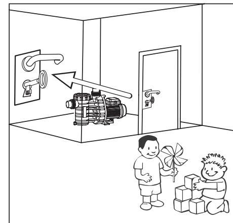
Ensure the motor's cooling. The installation site must be dry and well ventilated. Never obstruct the air supply to the fan by putting any objects on the pump or too close to the pump.
