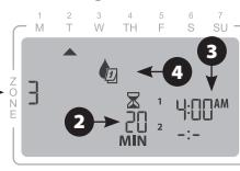
**2 Set Watering Run Time:** Press + or - to set desired RUN TIME; then press NEXT.
