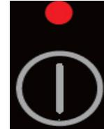
3. A red-light indicator will be on when the glass is still hot. It will disappear when the surface has cooled down to a safe temperature.
