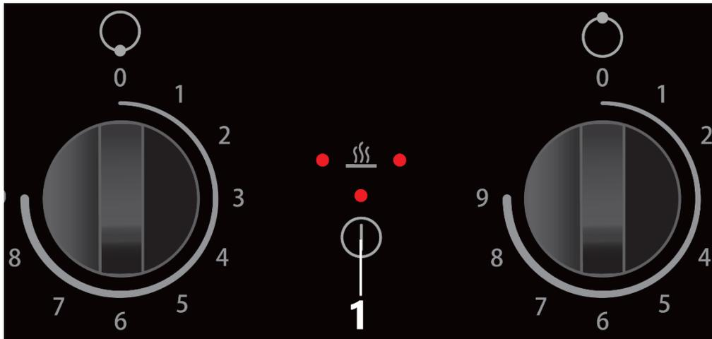
1 | Sensor buttons for turning the hob ON / OFF
