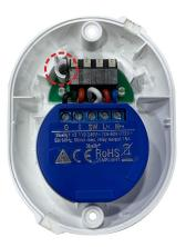
Place the button extension lead, as shown on the picture above.
