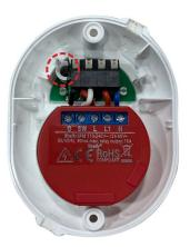
Place the button extension lead, as shown on the picture above.
