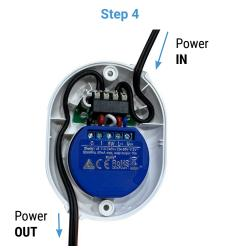
Inside the case of Shelly Button there are guiding arrows, which show how to organise the power cables. After placing the cables, they should look as shown on the picture above.
