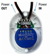
Connect the power (input and output) cables, as shown on the picture above.
