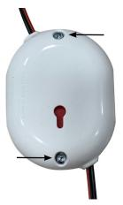
Put the screws in the holes, shown on the picture above and tighten the top and botton parts of Shelly Button.
