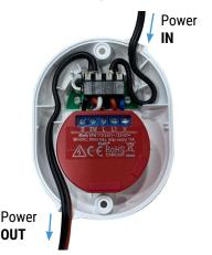
Inside the case of Shelly Button there are guiding arrows, which show how to organise the power cables. After placing the cables, they should look as shown on the picture above.
