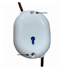
Put the screws in the holes, shown on the picture above and tighten the top and botton parts of Shelly Button.
