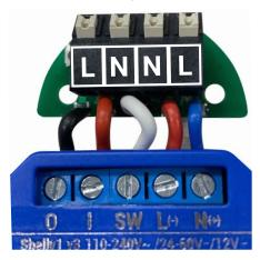
Connect the wires, as shown on the picture above.
