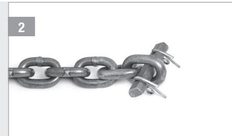
3 To indicate the wear of the load chain, measure the load chains link  $\varnothing$  and the inner length of 5 chain links regularly:
