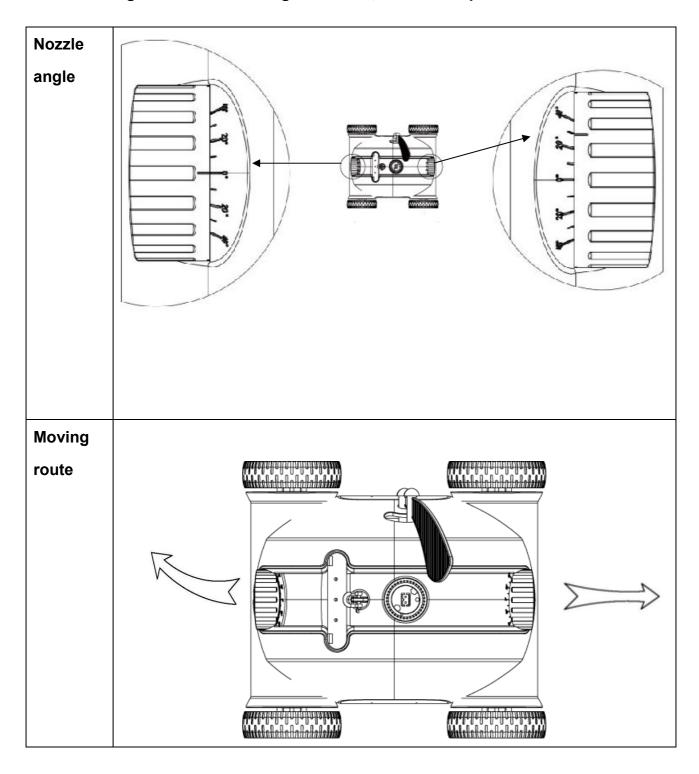
Setting Two: 0°——40°, when the cleaner does not have a full coverage of pool.
