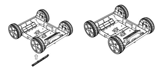
c. Please ensure that top cover of the cleaner is tightly assembled with its chassis.
