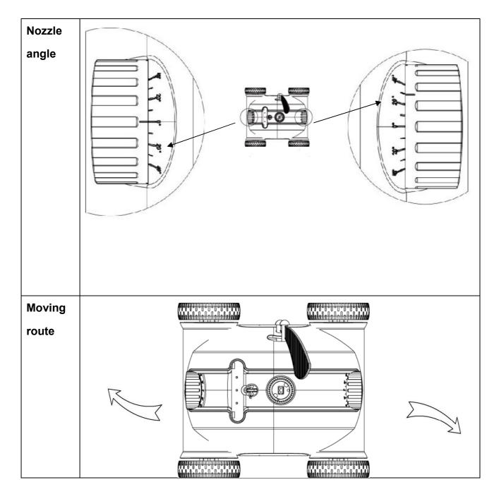
Note: above are recommended settings and different settings might apply to specific pools. So the operator can set according to the principle of nozzle settings and the actual situation of the pool.
