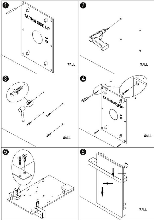
1. Use the supplied template to mark the position of the holes on the wall.
