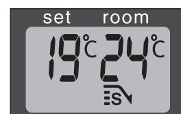
J: When the SAVE light lights up, the heater will automatically switch on or off in order to remain within a specified temperature range.
