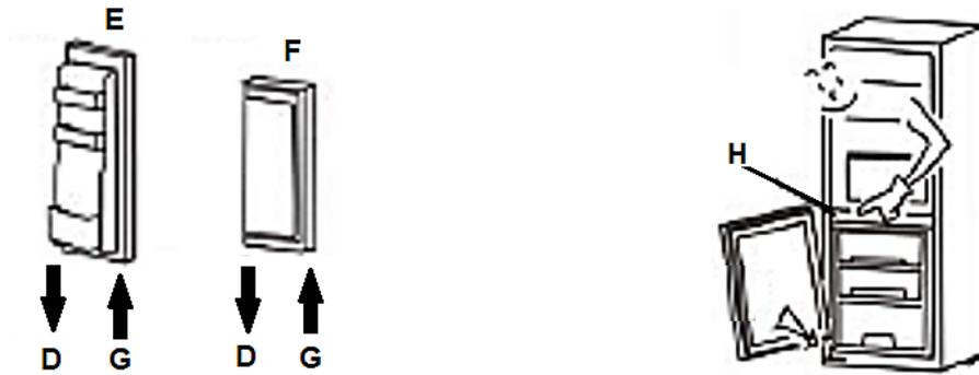
7. Place the fridge-door on the middle hinge; the hinge pin must be inserted in the hole on the bottom of the fridge-door. Close the door, then install the top hinge on the opposite side. The top hinge pin must be inserted in the hole on the top of the fridge-door. Install the hinge cover.
