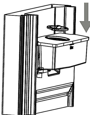
6. Check that the water tank is properly seated in the appliance door.
