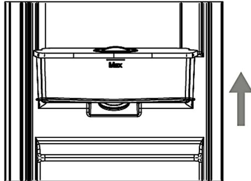
3. Remove the cover of the water tank (s. fig. on the right).
