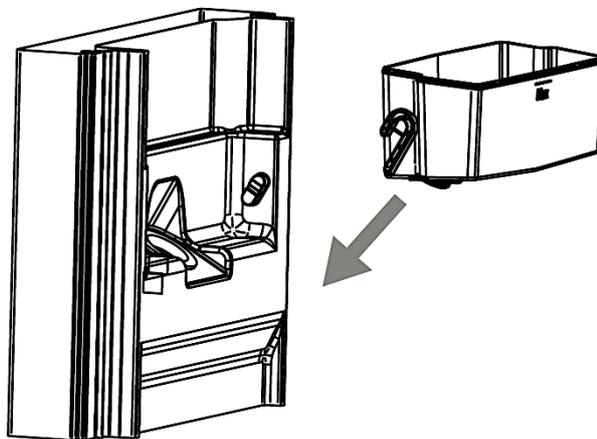
2. Install the cover of the water tank properly (s. fig. on the right).
