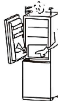
**NOTICE!** Adjust the doors properly. The seals must close properly.
