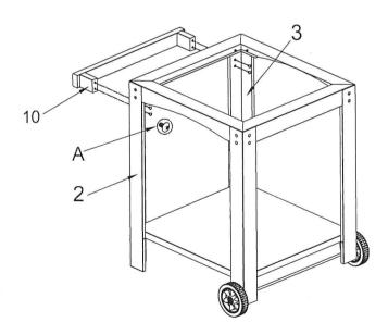
Slide the Side handle (10) onto Left front leg (2) and left back leg(3) with four M6\*12 screws(A) tighten by hand.
