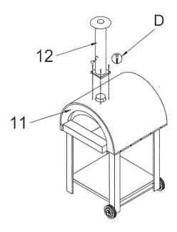
Slide the chimney assembly (12) onto firebox assembly(11) whit four M6\*38 screws(C) tighten by hand.
