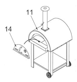
Slide the door assembly (14) onto the corresponding position of the firebox assembly(11)
