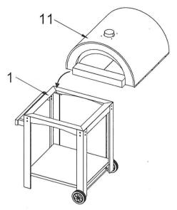
The firebox assembly (11) is lifted and onto the corresponding position of the frame roof(1)
