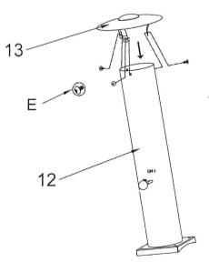
Slide the chimney cover (13) onto the chimney assembly(12) with three M6\*12 screws(E) tighten by hand.
