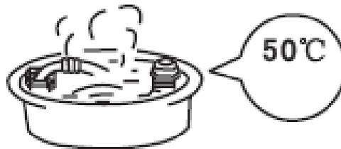
5. Pour warm water (2 - 3 litres / approx. 50 °C) into the drum and wait approx. 10 minutes (s. fig. below).
