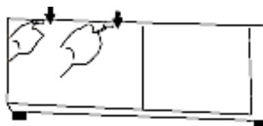
2. Open the locks and remove the condenser.
