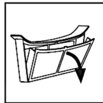
4. Clean the fluff filter. Remove any contamination with a damp cloth
