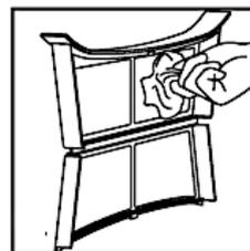
6. Insert the fluff filter properly (**the fluff filter must be dry completely**).
