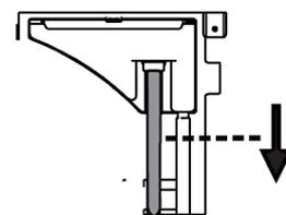
2. Connect the water drain hose of the appliance to the external water drain hose.
