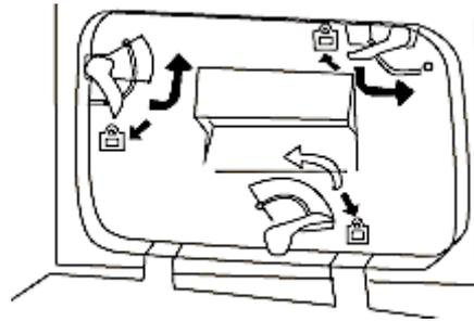
3. Remove the fluff. Clean the condenser carefully using a clean brush.
