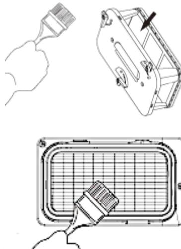
4. Reinstall the condenser properly and close the locks. **The condenser must be completely dry before reinstallation.**
