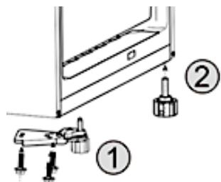
14. Install the assembled lower hinge unit to the lower left side of the appliance (see fig. on the left, 1).
