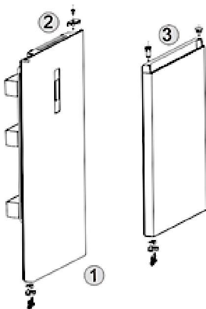
16. Take the left stopper (plastic) from the accessory bag, place it on the other side of the door together with the metal stopper removed from the right side and fix it with two screws (see fig. on the left, 1).
