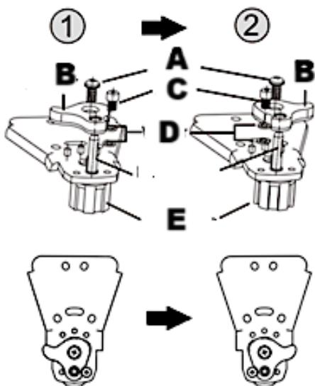
12. Uninstall the lower hinge: Remove the fastening and the hinge pin of the lower hinge assembly one by one. (see fig. on the left, 1).
