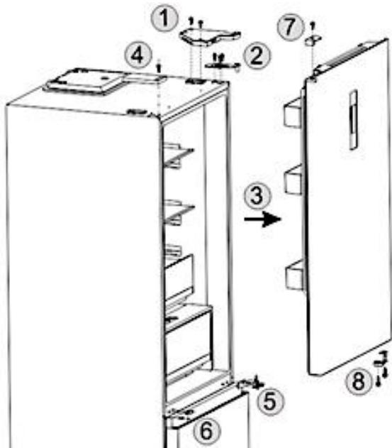
1. Unscrew the upper door hinge cover and remove the door hinge (see fig. on the left, 1).
