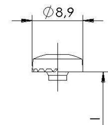
Pan head with and without milling ribs underneath the head
