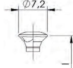
Raised countersunk head 90° with and without milling pockets
