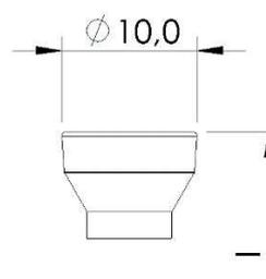
Cylindrical head with counter-sinking
