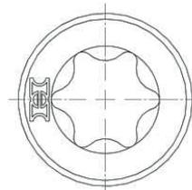
Head markings for  $d = 4,5$  to  $10.0$  of types: Cylindrical head, cylindrical head with countersinking.
