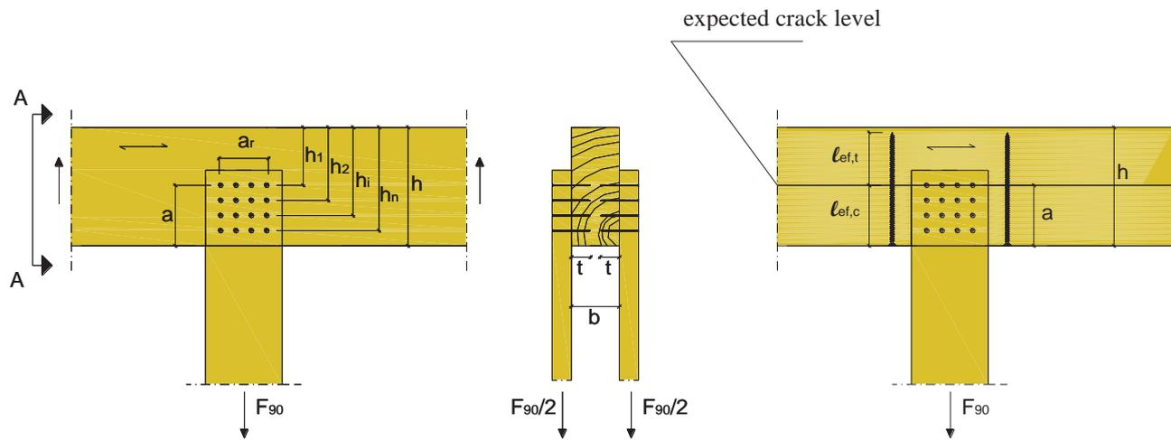
Figure 5: Example for tensile reinforcement of a connection force perpendicular to the grain
