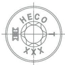
Head markings for  $d = 6.0$  to  $10.0$  of types: flat countersunk head.
