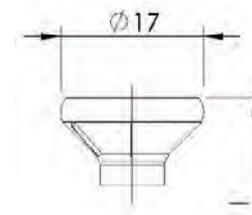
Flat countersunk head, with and without milling ribs
